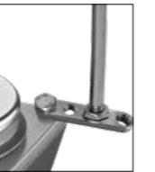
Note: When using bath attachments with a diameter over 180 mm, please use support rod in conjunction with an extension. (See "Accessories")
